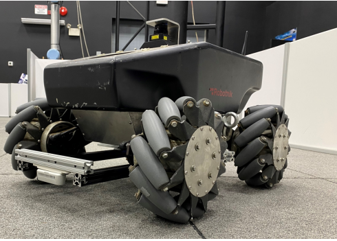
Fig. 1: A downward facing camera setup configured by the authors. Note this is not the one used for gathering the experimental data considered in this paper, but is illustrative of a typical setup.
