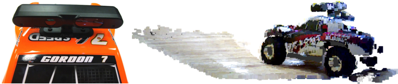
Figure 4: (Left) The Asus XtionPro RGB-D sensor is mounted on the roof of the RoSCAR shell. The sensor provides 640 x 480 points at 30 fps (Right) Visualization of 3D point cloud with RGB color registered to each point, taken from the view of a racing RoSCAR. Here, a second RoSCAR can be seen.
