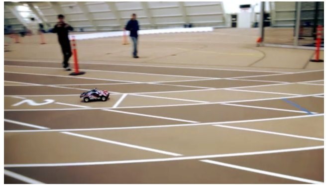
Figure 6: (Left) A view from Rauch Field House. Total track length around the course was 200 m, which is appropriate for the scale of the RoSCAR. (Right) Extraneous markings on the Rauch track necessitated robust solutions to lane segmentation and tracking.
