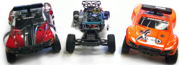
Figure 1: Three RoSCAR platforms pictured with and without shell attached. The only external distinguishing feature is the RGB-D sensor mounted on the roof (left and right cars). Internally, a mini-ITX x86 computer is mounted to the chassis, along with servo control, encoder, and multiplexer hardware (center car).
